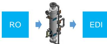
The goal is to reduce CO<sub>2</sub> content before EDI to less than 5 ppm. Operation mode is air sweep.
