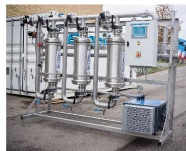
*Case: Membrane degassing unit in combo operation mode for removal of oxygen to less than 20 ppb. Complete frame-mounted solution with control panel and vacuum pump. The application is boiler feed water.*
