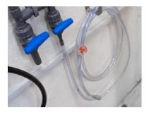
Tapping equipment with two outlets. One is fitted with a hose with automatic stop function ensuring the correct volume of water for your battery.
