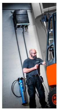
A quite simple solution for production of battery water comprises a SILEX unit, a water tank, and tapping equipment.
